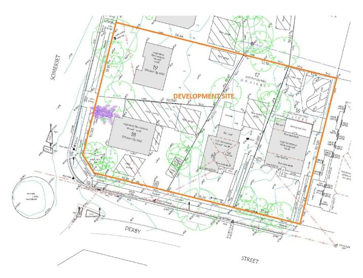
The total site area for the four existing lots is 2343m2 (less than 2500m2). The survey plan indicates an existing 675mm diameter council drainage pipe is located parallel to the Derby Street frontage and affords the opportunity for an underground stormwater connection with the provision of a new kerb entry pit.
